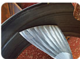
Figure 3. Coating Kort nozzle barrels with a thermally applied spray coating can eliminate the gap between the propeller blade tips and the wall of the Kort nozzle barrel, thereby making the nozzle more efficient.
