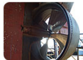
Figure 2. A Kort nozzle provides increased control of the water turbulence passing through it.
